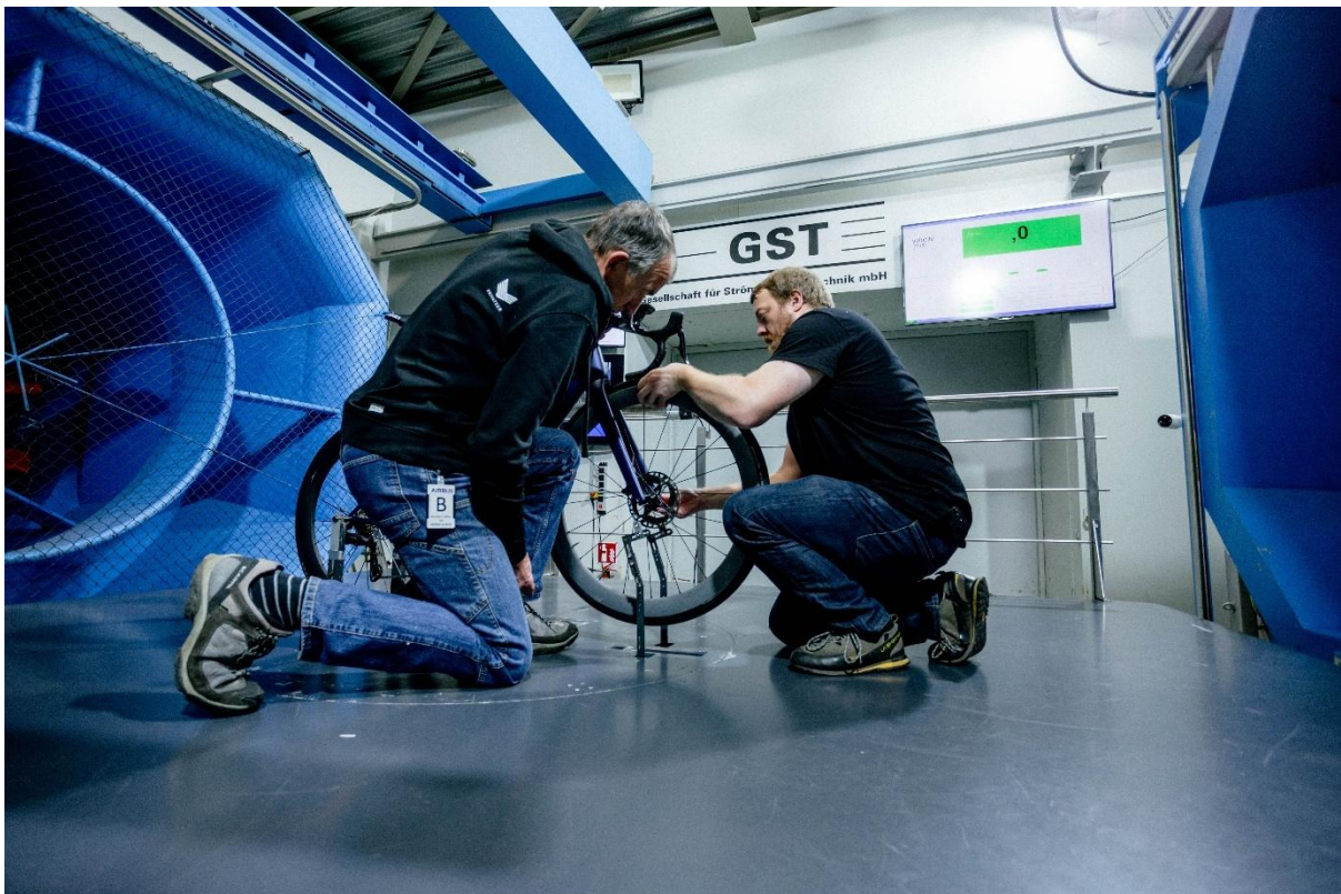
Figure 2 - 3D printed prototype being fitted to test bike at GST tunnel
