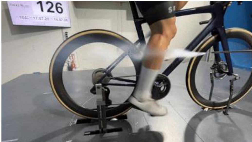
Figure 9 - Smoke visualisation of the drag introduced by a rider's leg
